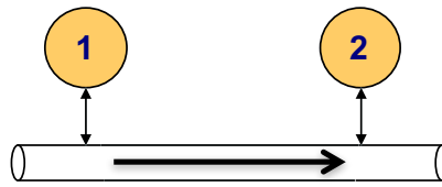
Figure 7: Schematic showing the basic setup of a cascaded quantum system, where two quantum systems interact via a unidirectional (i.e. “chiral”) waveguide. In the Markovian limit, the interactions mediated between the two systems via the waveguide correspond exactly to our effective directional Lindblad master equation.
